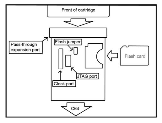
If you are using the pass-through expansion port, mind the correct orientation of the card! On a C64/C128, the side that normally faces up (label side) must face to the user. On an SX64, the label side of a cartridge in the passthrough port must face down.
