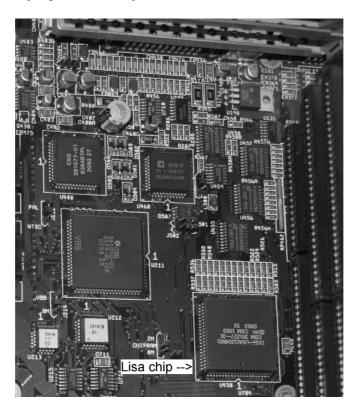
The picture above marks the Lisa chip, which is responsible for the video output of the Amiga. The socket of Indivision AGA MK2 is placed over top of this chip. The connector for the cable of Indivision AGA MK2 must face to the mouseports.
