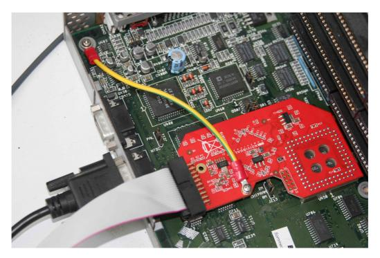
We recommend using the included grounding cable. If you connect the cable as shown in the picture, please make sure that the washer has direct contact with the flickerfixer board. Also, please make sure that the cable does not cause a short with nearby components. Now you can put any Zorro cards back into the slots. For better ventilation, it's a good idea to have a short board in the lower slot.
