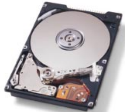
IBM Travelstar 20GN 9.5 mm 4200 RPM, 20 GB ATA-4 hard drive
